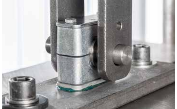
Tensile testing of the STAUFF Bond Plate (type SBP) with adhesive (type CB420-50E)
