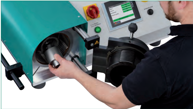
Insert the tube shaper into the tool holder of the machine and use the bayonet lock to secure it.
