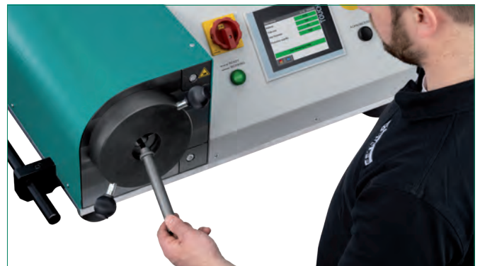
Remove and visually check the formed tube end.
