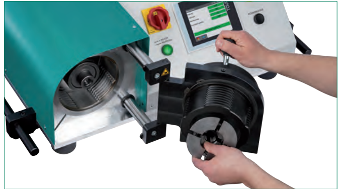
Insert the clamping jaws into the clamping head of the machine and push them completely in until it stops.
