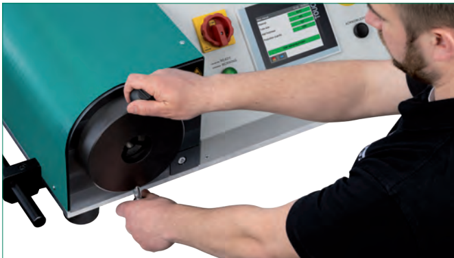
Close the clamping head, push it into the machine and lock it by turning in clockwise direction.
