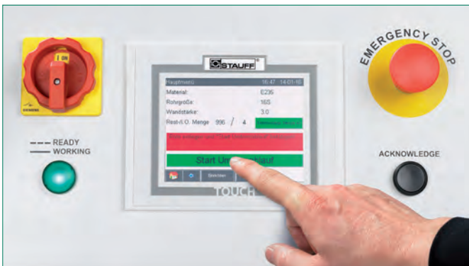
Use the operating panel to start the actual forming process.
