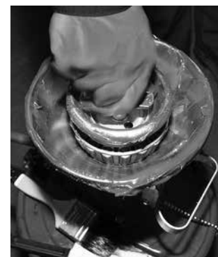
Fig. 22. Mechanical grease packer.
