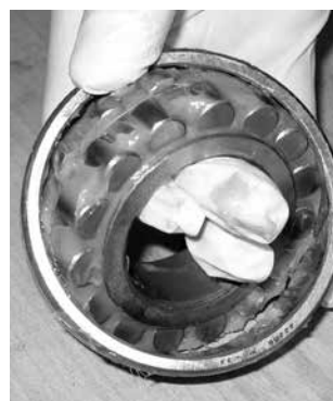
Fig. 21. Grease can easily be packed by hand.
