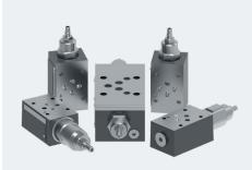
These compact hydraulic systems feature modular valves that are "sandwich" mounted between a directional control valve and a standard mounting surface. All circuit flow paths are contained within the control valve and modules. These valves provide a compact hydraulic circuit at a reduced cost, eliminating interconnecting piping. Each valve "stack" can be configured to provide the specific system functions.
