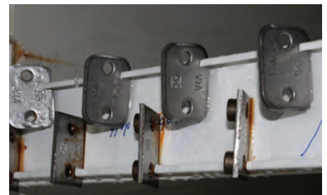
Salt-spray testing of ACT Mounting Hardware (above of the picture) compared to contaminated hardware made of Stainless Steel V4A (below of the picture)
