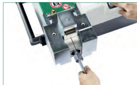
Tooling head for 37° tube flaring based on settings manually defined by the operator
