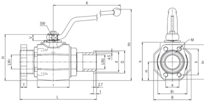
**High-Pressure Forged Body Ball Valve ■ Type FBV-2-F/C3**
