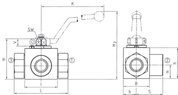
**High-Pressure Block Body Ball Valve ▪ Type CBVL-3
