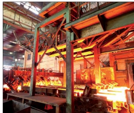
**Descaling of steel sheets and profiles.**
