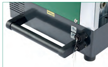
Connections for the tool head as well as for the external foot control switch
