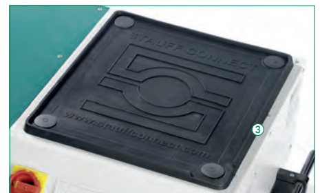
Noise-reducing tool tray with durable rubber mat
