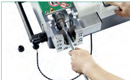
Tooling head for cutting ring assembly based on pre-defined settings / automatic tool size detection
