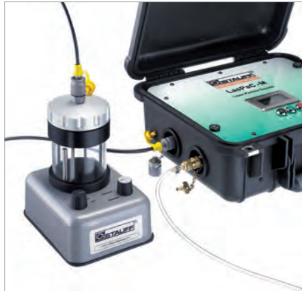
LasPaC-II-M with small Bottle Sampler
