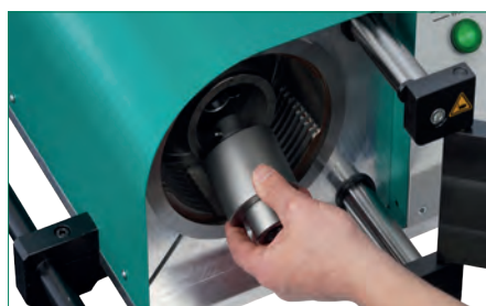
Inserting the tube shaper into the tool holder – with no tools required
